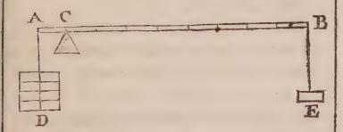
Where suppose the Leaver to bee represented by the length AB, the center or \* prop at the point C, the weight to bee sustained D, the powerthat doth uphold it E.
